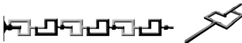
Fig. 4. Scheme of “split-and-recombine” mixing within three-dimensional, G-shaped microchannels.
